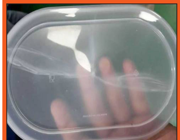
Dyna-Purge A successfully purged fluorescent coloured Polypropylenes.
