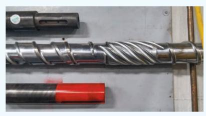
Large blow molding machines at ThermoFisher Scientific's Rochester, N.Y., facility routinely use Dyna-Purge F2 product for cleaning heads and extruder screws. ThermoFisher molding personnel say this practice reduces black-speck contamination after the machine comes out of a scheduled shutdown. Recommended purging procedures outlined in this article deliver significant time savings and reduce resin waste during startup, says ThermoFisher.
