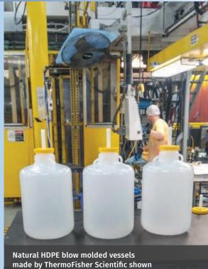
made by ThermoFisher Scientific shown here are finished with injection molded closure.
