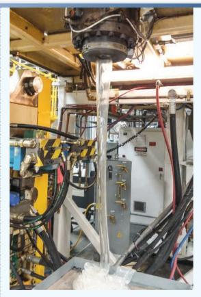
The value of purging is especially beneficial when shutting down for an extended amount of time, like a weekend. Thermo Fisher fills the barrel with Dyna-Purge to prevent oxidation, a major cause of degradation. As the machine cools, Dyna-Purge will solidify and shrink, pulling residue away from the barrel walls.
