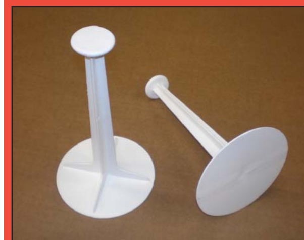
Plungers – first shot after purging with Dyna-Purge M (no discoloration/streaks from Black to White colour/material changeover)
