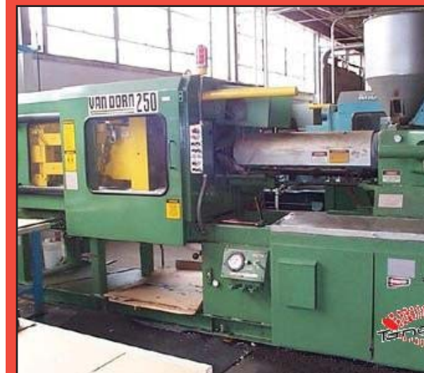
Just 3 kg of Dyna-Purge M is required to purge the Van Dorn 250 machine versus 20 kg of the previous purging materials.
