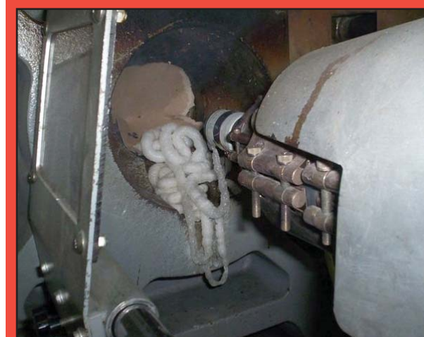
Purging with Dyna-Purge requires just 3 pounds of material versus 6 pounds of the clear polystyrene used in IMCO's previous purging methods.
