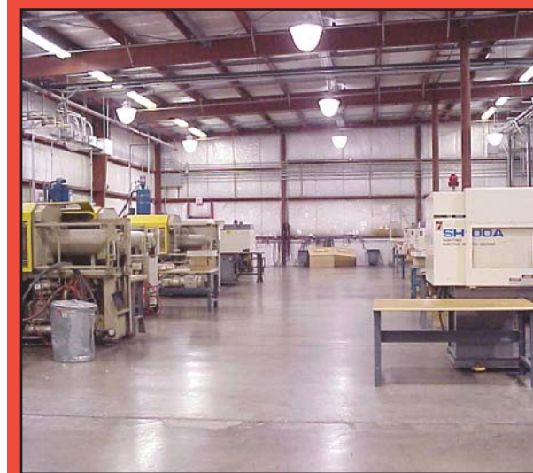
IMCO's 28,500 square foot facility features a variety of injection molding presses ranging from 40 tons to 720 tons
