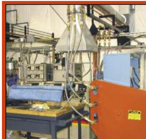
Reynolds Packaging's R&D facility operates a single screw extruder with a flat coat hanger die.
