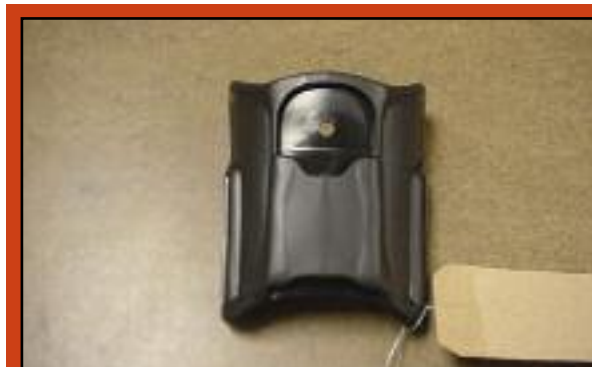
Transitioning from this black PC/PBT part to grey PC proved to be challenging. Ultimately, Dyna-Purge® M worked faster and more effectively than regrind.
