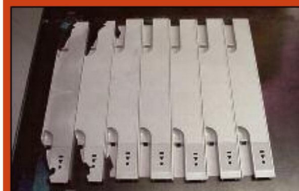
After using Dyna-Purge® M, Duramould was able to transition to a light grey PC in only 7 shots.
